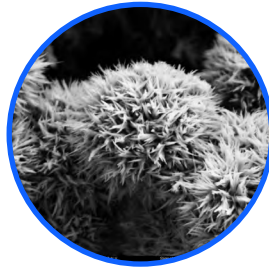
Hydroxyapatite formation of ProRoot® Bio Sealer 2
